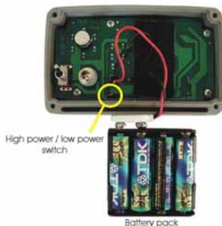
Figure 2: Infrared lap transmitter HIGH/LOW power switch
